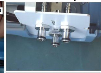
Note: Make sure "A", "B" and "C" ports are tightened properly. Use the deep socket (spark plug) wrench to tighten all ports on the end plate.
