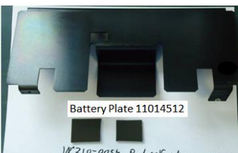
Use scissors to cut 2, 31mm x 31mm square pads from part number 210-0054.
