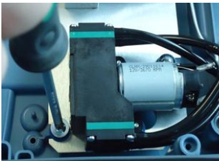
Obtain the Rear Housing enclosure and align and place the solenoid pump assembly on the bosses of the housing enclosure to tighten.
